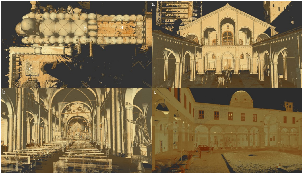
Fig. 9 Laser scanning data: point clouds of: a) the Quadriportico; b) the Basilica; c) the Rectorio designed by Bramante.
