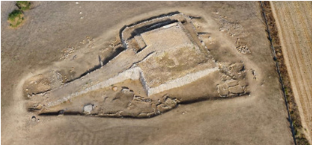
Fig. 7 Mesh processed from the point cloud of the photogrammetric survey (graphic elaboration by Andrea Sias, GRA-VIS LAB - Laboratory of Graphic and Visual Sciences).
