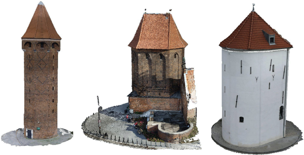
Figure 11 Structure from Motion models of fortified towers in the city centre. Data elaboration by D. Bursic and P. Giardini from Metaheritage enterprise.
