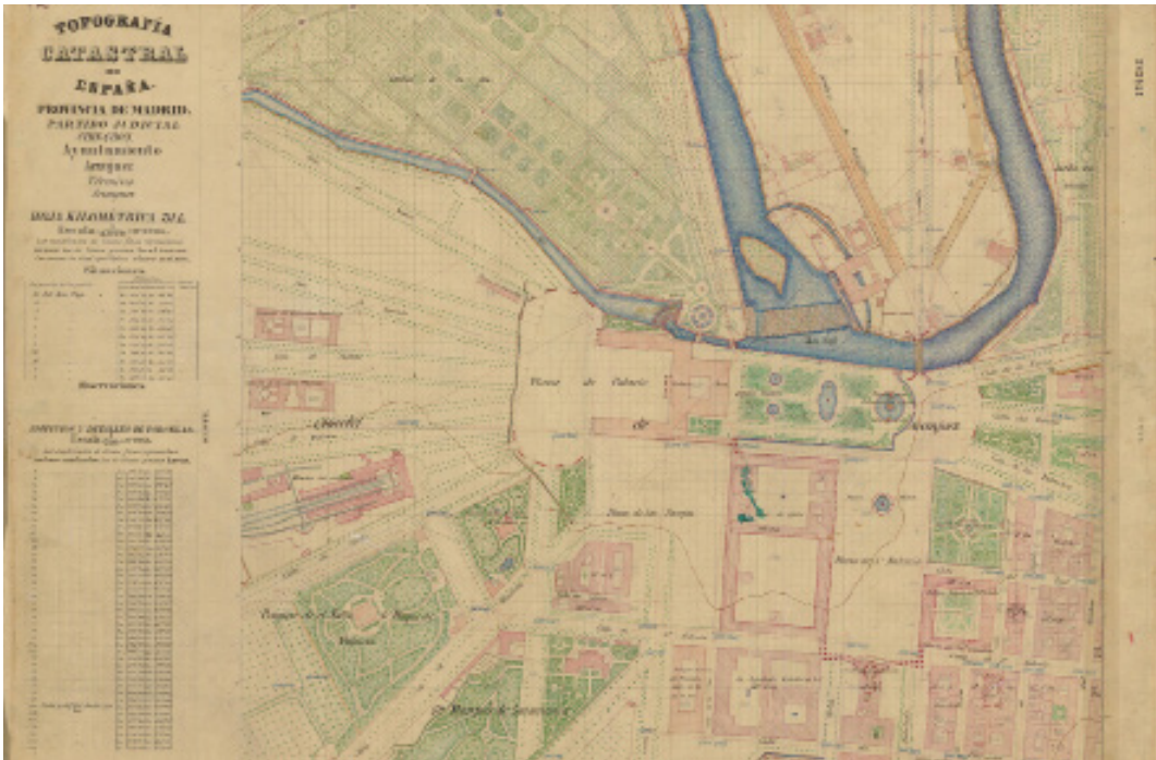
Fig. 6 Junta General de Estadística 1860-1870, Topografía Catastral de España, Catastro de rústica, Hoja Kilométrica 31L (Aranjuez). Instituto Geográfico Nacional, Madrid, Spain. This set of maps 1:2,000 was produced according to the highest standards of accuracy. The project included the related cadastral information of each plot. Although unfinished, the project is still an outstanding source of geographic, rural and urban information of the Spanish territories in the mid-nineteenth century. The set of their first drafts is still preserved. It served as the basis of the National Topographic Map ( Mapa Topográfico Nacional , MTN) of Spain 1:50,000, that was produced two decades later.
